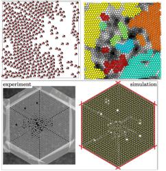
Self-propelled hard disks describe the motion of vibrated polar grains, a model experimental system for dry active matter.
